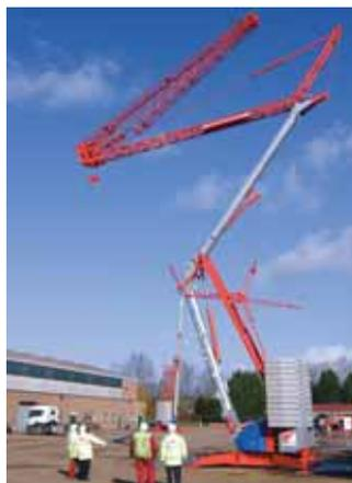
Kier Plant has added a contingent of self-erecting remote controlled cranes to its growing fleet. The Potain Igo 50s have a maximum jib length of 40 metres and can lift up to four tonnes. These electrically-operated cranes are clean and quiet to run and are used mainly on small, low-rise residential and brownfield sites where space is restricted.
